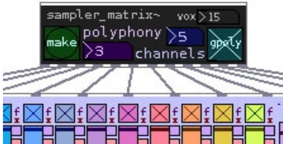
Figure 5. The sampler_matrix~ is a self-configuring polyphonic sampler.
