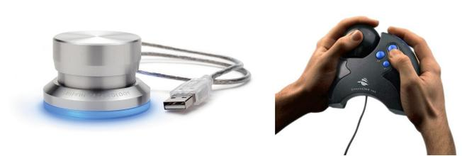
Figure 5: PowerMate USB knob and SpaceOrb
